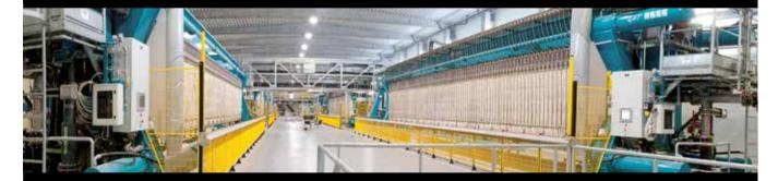
With its unique overhead beam design and four pull-to-close hydraulic rams, the GHT 4X4 outperforms all traditional filter presses through superior capacity, efficiency and reliability. It is fully automatic and designed to dewater large volumes of slurry with maximum speed and efficiency.
