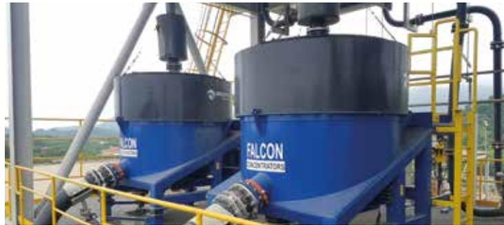
*Sepro's Falcon C gravity concentrator is capable of collecting fine minerals that would be missed by dense medium separators, spirals and other low G processes*
